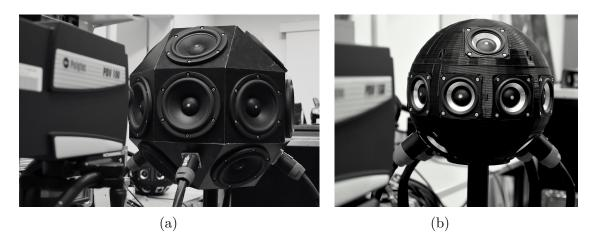
Figure 4.4.: MIMO voltage-to-velocity measurements with a laser-doppler vibrometer aiming at the center of a loudspeaker cone. All loudspeakers are excited with an exponentially swept-sine and the crosstalk is measured at the loudspeaker the LDV is aimed at.
