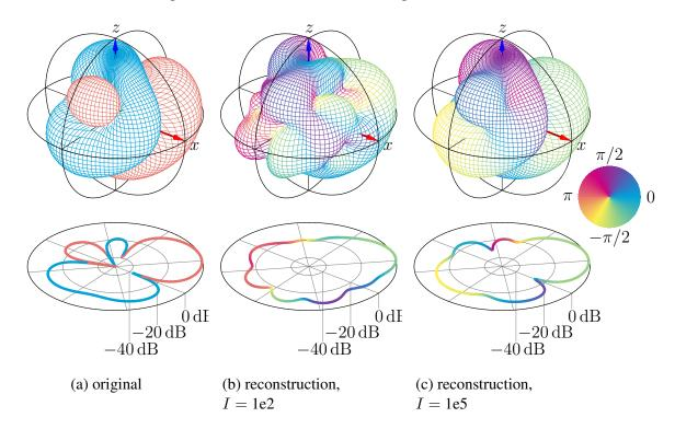
Figure 3.5 – Reconstruction of a random directivity function (L = 2) from 64 magnitude points with gradient descent algorithm for different numbers of iterations *I*. The initial phase is random.
