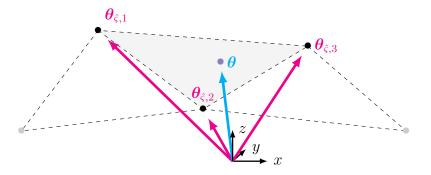
Figure 2.2 – Sample configuration for a virtual microphone at  $\theta$
