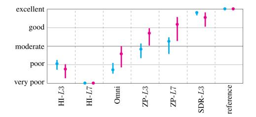
Figure 5.8 – Perceived quality of the radiated signal in reverberant environment for different positions. The large points depict the estimated median and the whiskers depict 95% confidence intervals of the median. → Position A → Position B.
