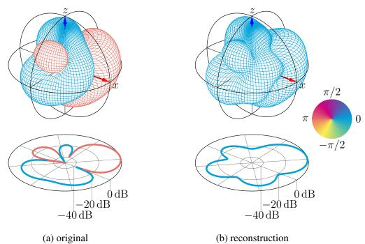
Figure 3.3 – Reconstruction of a random directivity function (L = 2) from 64 magnitude points with the zero phase method.
