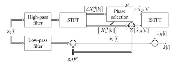
Figure 2.3 – Interpolation procedure from the signals of selected microphones subset with MVBAP.
