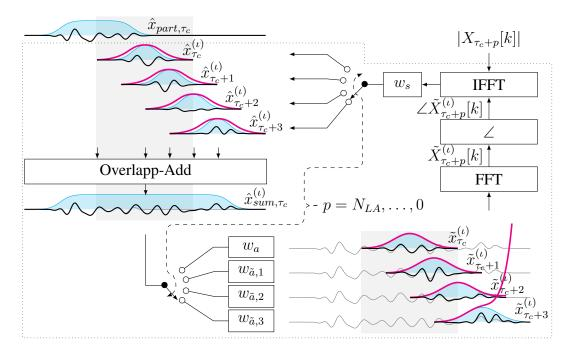
Figure 4.3 – Iterative phase estimation of time frame around  $\tau_c$  by mean of GSRTISI-LA. The cyan surfaces depict the effective windowing of the signal. The magenta lines depict the window applied by the previous processing block ( $w_a$ ,  $w_{\tilde{a},p}$  or  $w_s$ ). The dotted frame highlights the part altered by each iteration. Within each iteration, p changes decreasingly from  $N_{LA}$ to 0. The gray patchs show the region of the time-frame to be committed.
