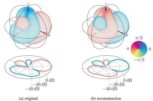
Figure 3.7 – Reconstruction of a random directivity function (L = 2) from 64 magnitude points with the SDR method using the main eigenvector and without further local optimisation.
