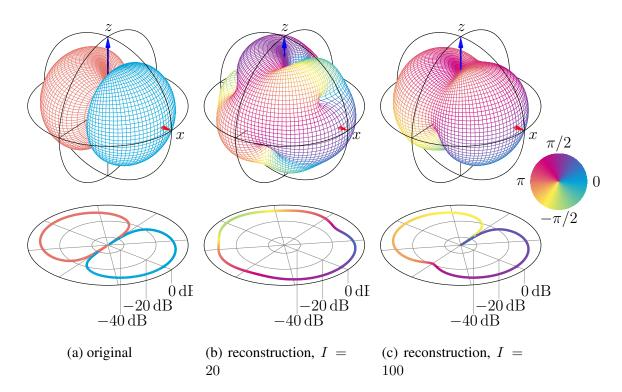
Figure 3.8 – Reconstruction of the dipole directivity  $Y_1^1(\theta)$  from 64 magnitude points by solving the MSLS problem with the Newton method.
