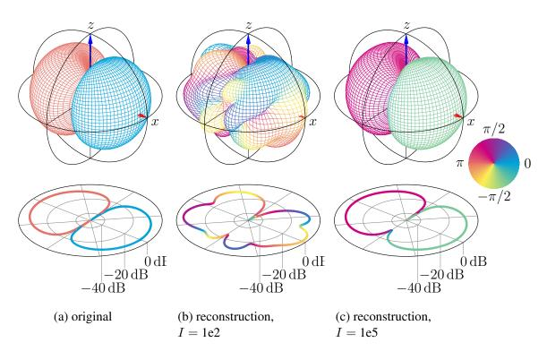
Figure 3.4 – Reconstruction of the dipole directivity  $Y_1^1(\theta)$  from 64 magnitude points with gradient descent algorithm for different numbers of iterations *I*. The initial phase is random.
