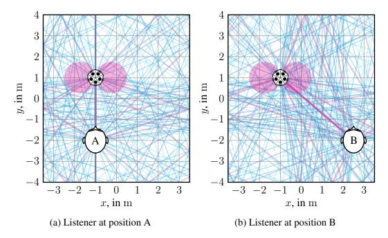
Figure 5.6 – Geometry of the virtual environment. The reflections are represented up to the  $5^{\text{th}}$  order.
