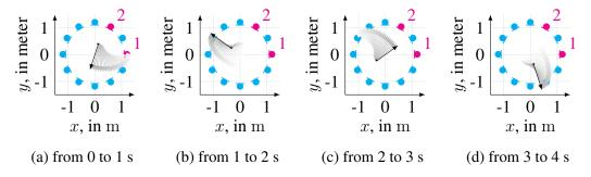
Figure 5.3 – Source movement used in the simulation. The source position defined a by 0.2 Hz anti-clockwise rotation on a centred circle of 0.4 m radius. The source orientation rotates in the clock-wise direction with a frequency of 0.3 Hz.
