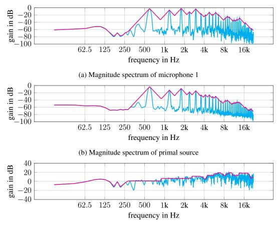
(c) Magnitude spectrum of radiation filter at the position of microphone 1
