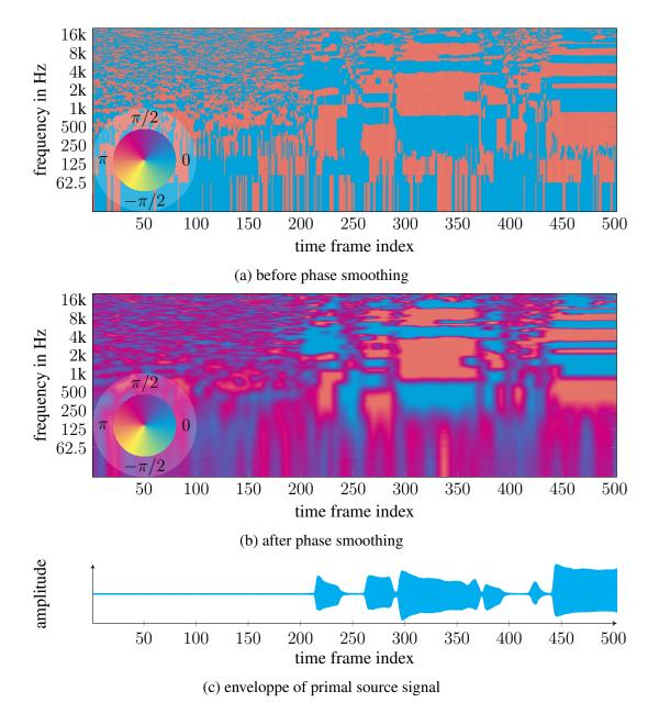
Figure 4.8 – Retrieved phase for microphone 1 from an alto saxophone recording by selecting the main eigenvalue of the SDR solution.
