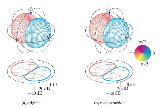
Figure 3.6 – Reconstruction of the dipole directivity  $Y_1^1(\theta)$  from 64 magnitude points with the SDR method using the main eigenvector and without further local optimisation.
