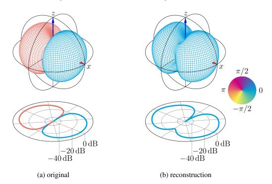
Figure 3.2 – Reconstruction of the dipole directivity  $Y_1^1(\theta)$  from 64 magnitude points with the zero phase method.
