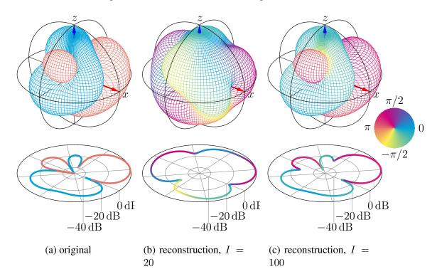
Figure 3.9 – Reconstruction of a random directivity function (L = 2) from 64 magnitude points by solving the MSLS problem with the Newton method.
