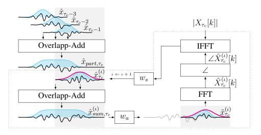
Figure 4.2 – Iterative phase estimation of time frame around  $\tau_c$  by mean of RTISI. The cyan surfaces depict the effective windowing of the signal. The magenta lines depict the window applied by the previous processing block  $(w_a \text{ or } w_s)$ . The dotted frame highlights the part altered by each iteration. The gray patchs show the region of the time-frame to be committed.
