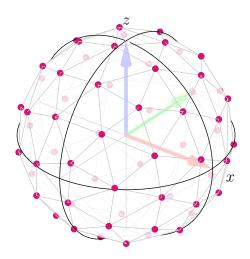
Figure 3.1 – Geometry of the IEM 64 microphones array
