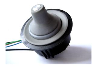
Figure 6.14: Assembled rotary encoder module
