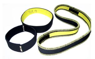
Figure 6.8: Neoprene belt prototypes
