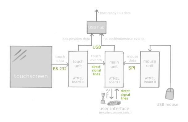
Figure 5.3: Hardware communication schematic
