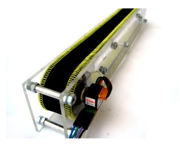
Figure 6.10: Optical encoder attached to pulley
