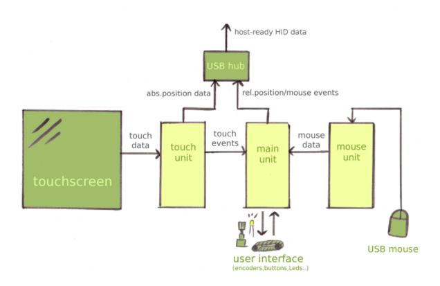
Figure 4.1: Schematic block diagram
