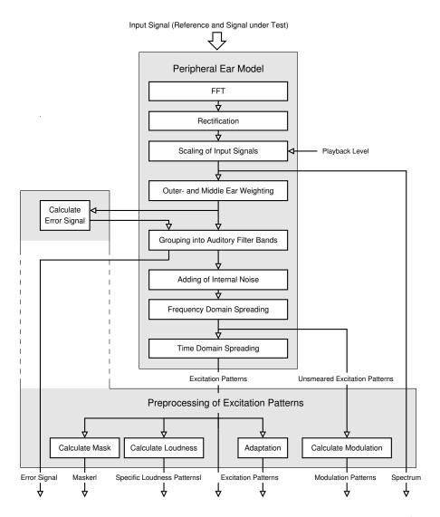
Figure 2.25.: FFT based ear model and preprocessing of excitation patterns (after [28])
