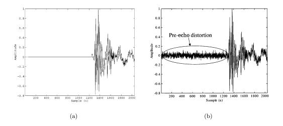
Figure 2.12.: Pre-echo example: (a) uncoded castanets and (b) transform coded castanets, 2048 block size
