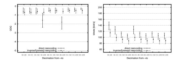
Figure 4.6.: Results for Vorbis decimation with settings quality 0.5, threshold -40dB, include boundary blocks.
