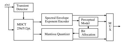
Figure 2.20.: AC3 encoder block diagram
