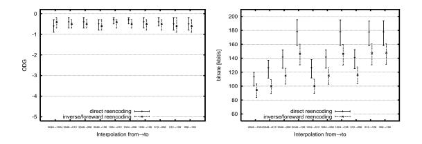
Figure 4.4.: Results for Vorbis interpolation with settings quality 0.5, threshold -40dB, include boundary blocks.
