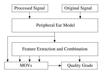
Figure 2.27.: High-level representation of the PEAQ model
