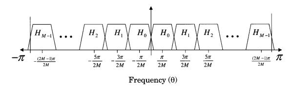
Figure 2.10.: Frequency response of the oddly stacked M-channel filter bank (from [2])
