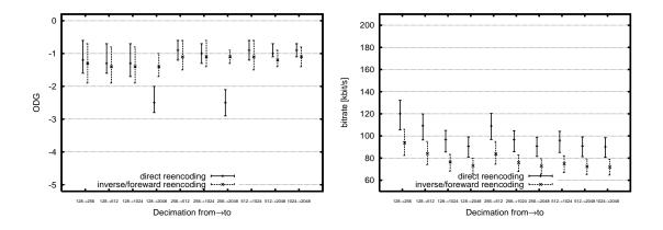
Figure 4.5.: Results for Vorbis decimation with settings quality 0.2, threshold -40dB, include boundary blocks.
