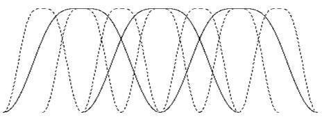
Figure 3.1.: Block sequence for changing the block length in MDCT. In this example the shorter block length is half the longer block length.
