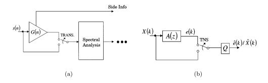
Figure 2.14.: (a) gain modification and (b) TNS scheme (from [2]
