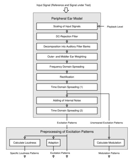
Figure 2.26.: Filter bank based ear model and preprocessing of excitation patterns(after [28]
