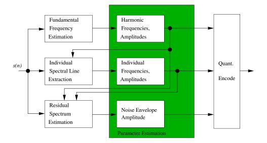
Figure 2.19.: MPEG-4 HILN Encoder Block Diagram
