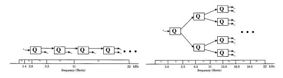
(a) Subband decomposition associated with a discreet wavelet transform
