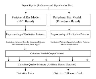
Figure 2.28.: Block diagram of the PEAQ advanced version
