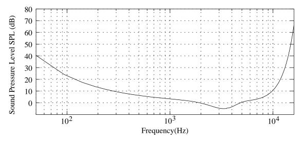
Figure 2.2.: Absolute Threshold of Hearing
