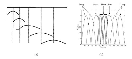
Figure 2.13.: Window switching: (a) Introduction of a transient window (center) to switch between two window lengths (from [9])(b) example window switching scheme (MPEG-1, Layer III) (from [9])
