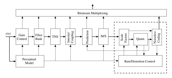
Figure 2.18.: MPEG-2/MPEG-4 Basic AAC Encoder Block Diagram
