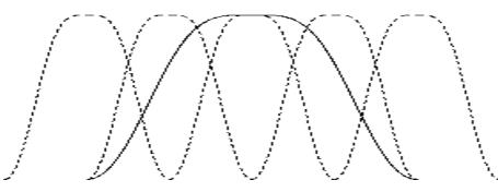
Figure 3.2.: Single long window with short window sequence of all blocks that contain data of the long window.
