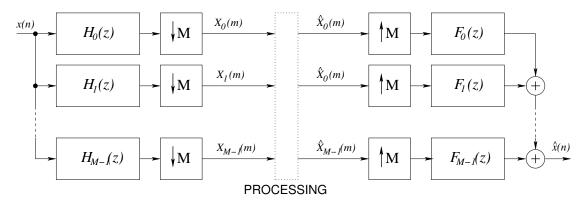
Figure 2.9.: Critically sampled M-channel filter bank
