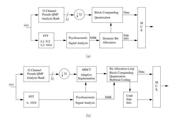
Figure 2.17.: ISO/IEC 11172-3 (MPEG-1): (a) Layer I/II encoder (b) Layer III encoder
