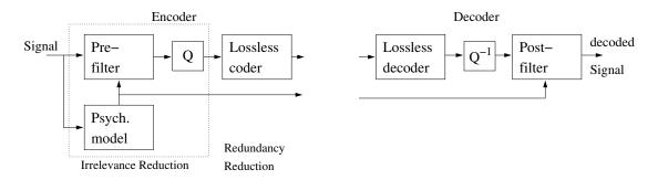
Figure 2.24.: Low latency coding scheme [23]
