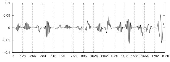
Figure 3.5.: Error signal for interpolation from 256 to 128 without boundary blocks for a male speech signal.
