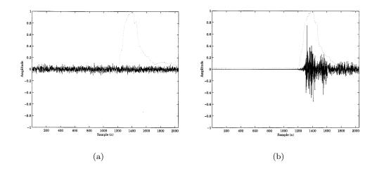
Figure 2.15.: TNS example showing quantization noise and the input signal energy envelope for castanets:(a) without TNS (b) with TNS (from [2]
