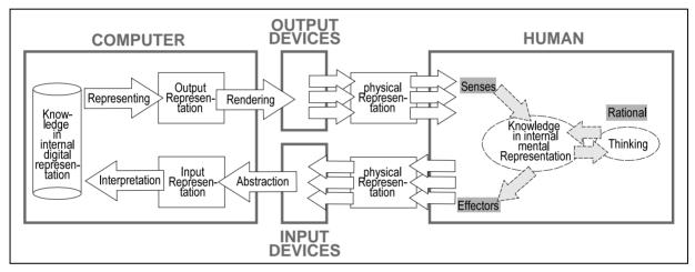
[Fig 8] Model for human computer interaction, after [12]
