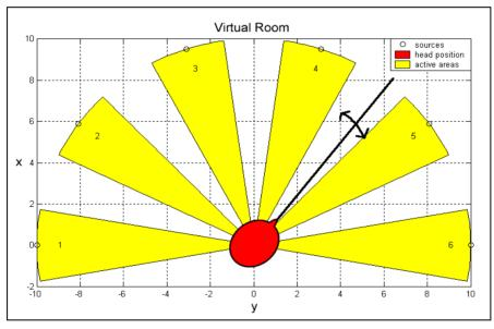
[Fig 13] Source positions and active areas within the virtual room
