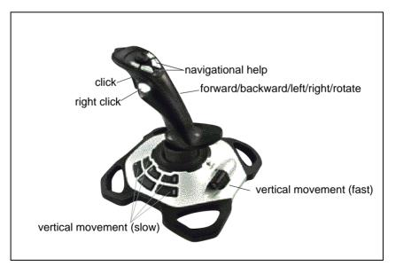
[Fig 18] Joystick with input possibilities
